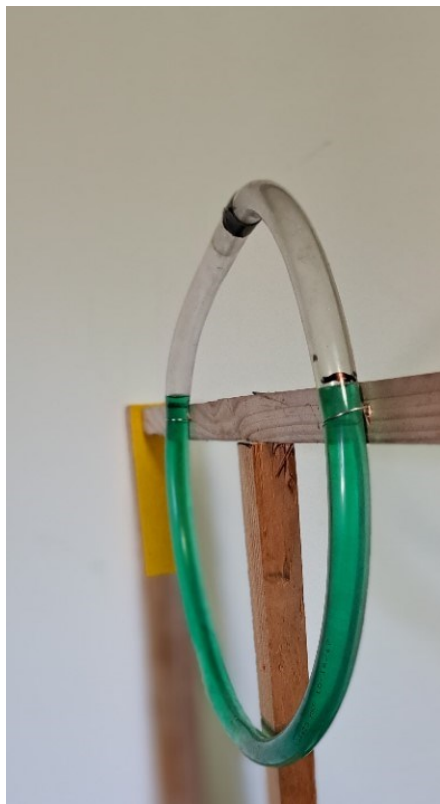
Figure 8 Surveyor will look along the cross piece (sight) and have the rod man move so that it is in line with the top of the cross piece.
