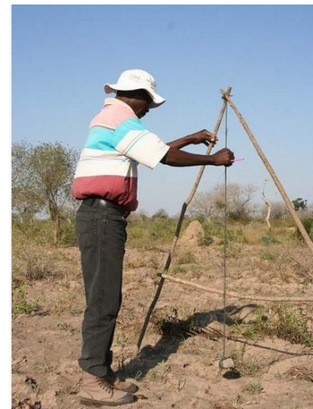
Figure 2. "A" Frame level
