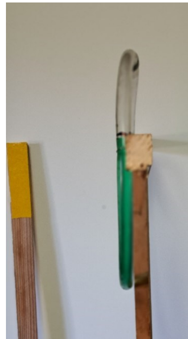
Figure 9. Looking down the sight piece with the top of water level matching top of sight. The sighting rod in the background with top level with top of sight
