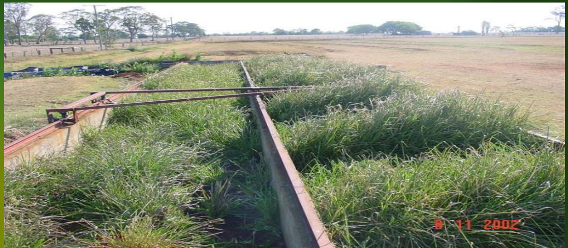
Hydraulic Flume: Two concrete testing channels, 2m wide and 20m long
