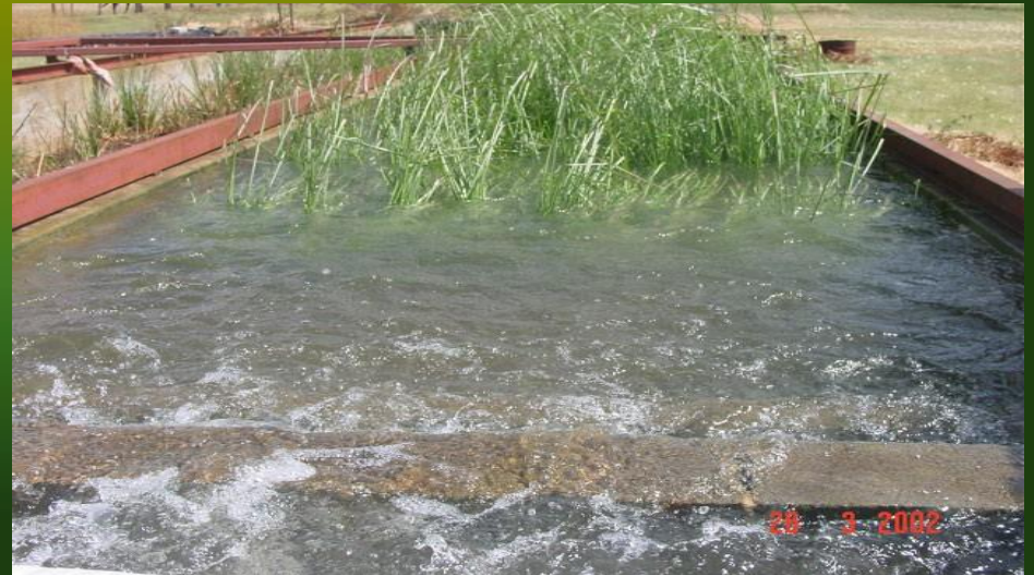
Hydraulic Flume: Two concrete testing channels, 2m wide and 20m long
