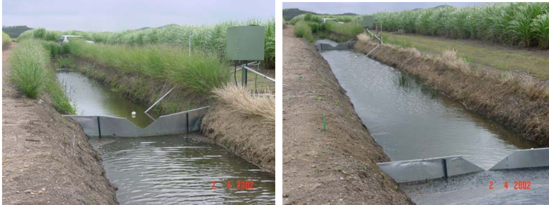
Fully instrumented experimental site with V notch weir to monitor volume flow. vetiver treated catchment LHS and control catchment RHS.
