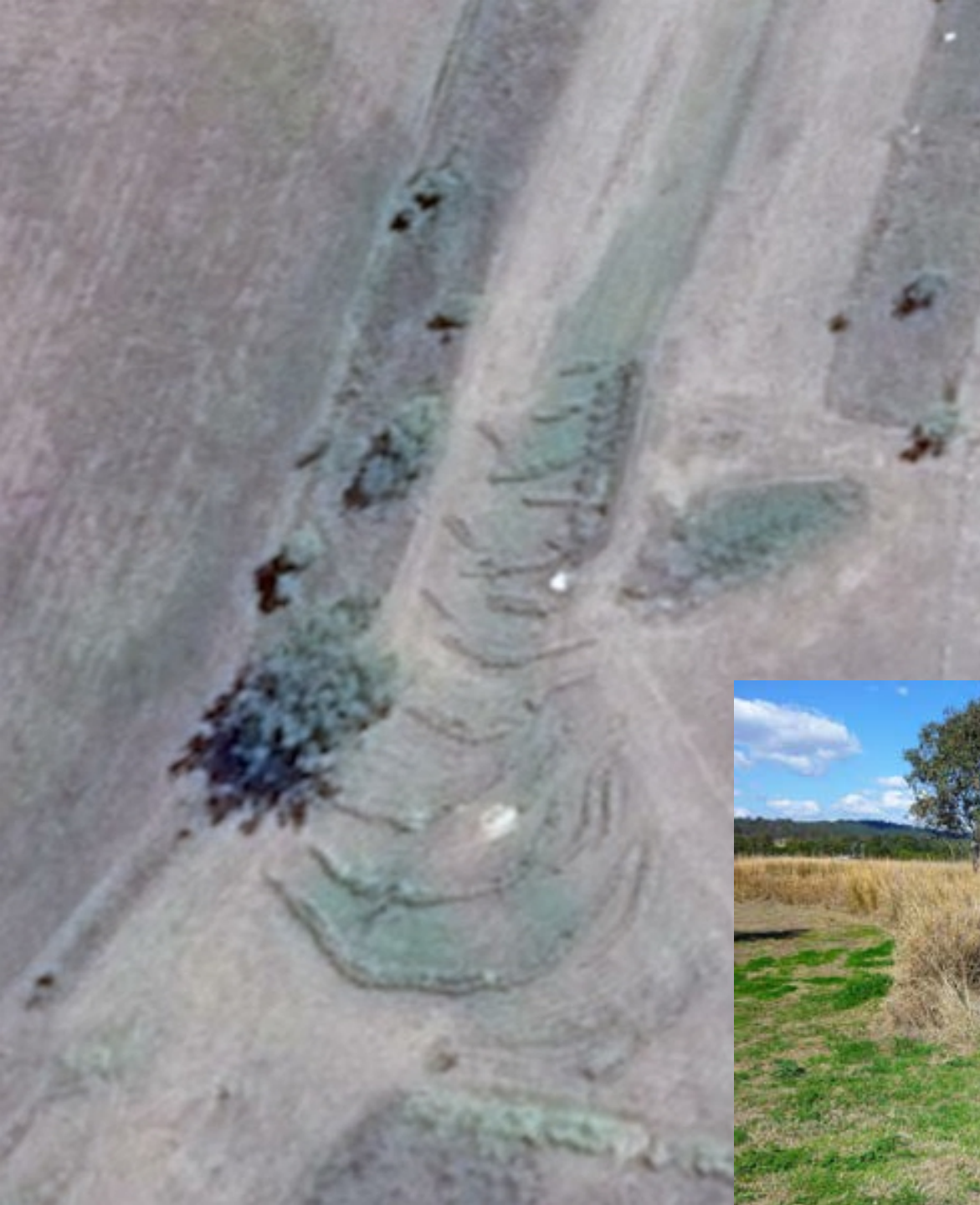
Vetiver hedgerows across major drainage channel (Storr's Creek) Laidley, Queensland, Australia. These hedges were subjected to major flooding and survived. Inset:Ground view
