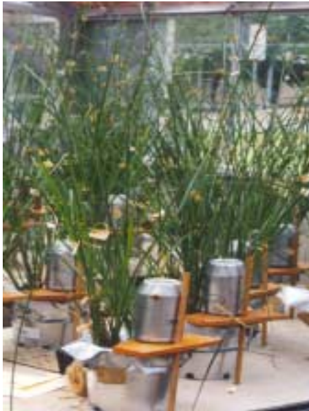
Plate 1: Pot set up displaying vetiver growing in 200 mm pots, with wooden stands and 1 L-reservoir bottles.
