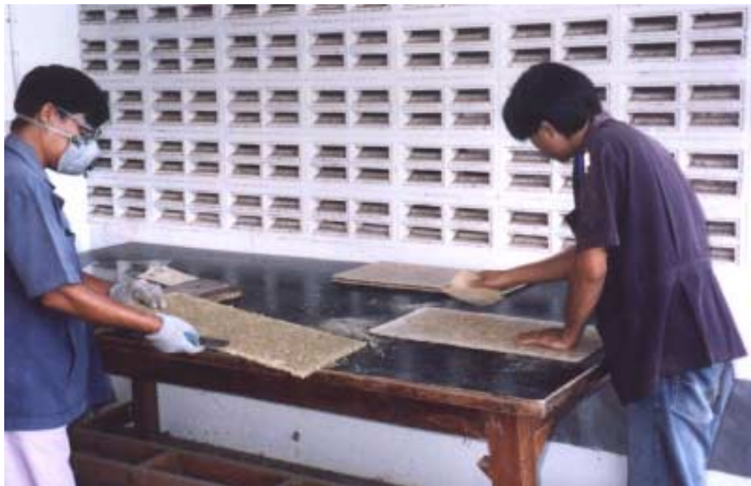
Fig. 25 Sample of Vetiver particle boards bonded by urea-formaldehyde; OHD and Phra Chom Klao Institute of Technology, Bangkok, 1999.
