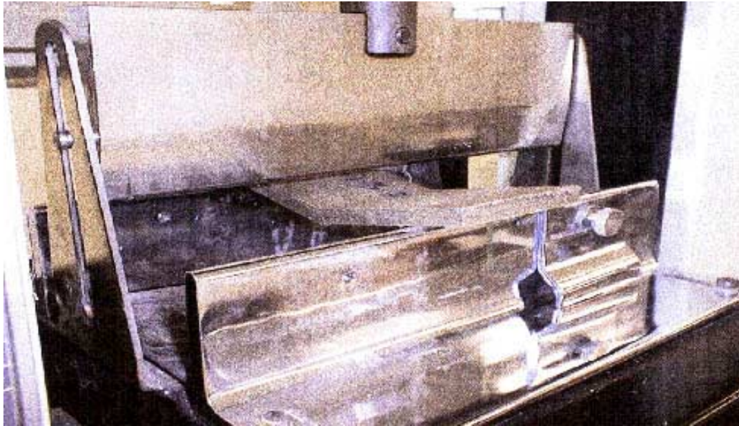
Fig. 28 Bending strength test for a Vetiver grass flake cement sample; Bangkok 1999.
