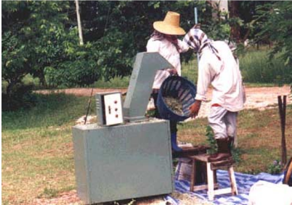
Fig. 30 A machine is under development for chopping stems, leaves or roots of Vetiver; preparing materials either for preliminary or exposure testing; Phra Chom Klao Institute of Technology, Northern Bangkok, 1999.
