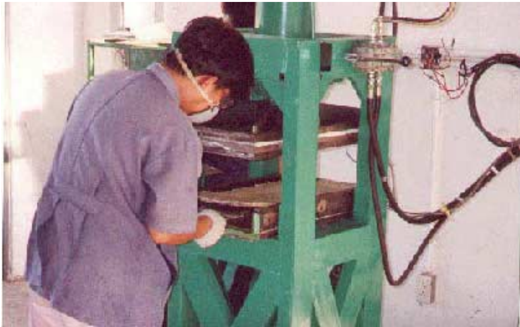
Fig. 24 Technical development for a Vetiver board bonded by thermal setting with urea-formaldehyde; OHD and Phra Chom Klao Institute of Technology, Bangkok, 1999.
