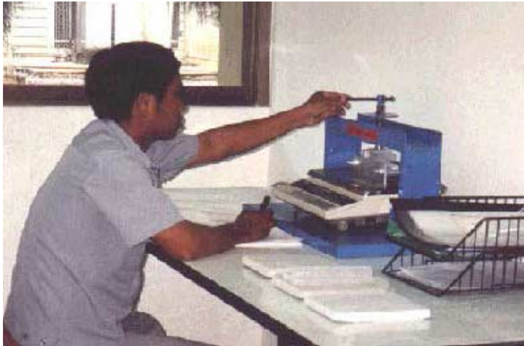
Fig. 22 Bending strength test for a Vetiver lightweight panel; TG Advance Center Co, Ltd., Lopburi, 1999.
