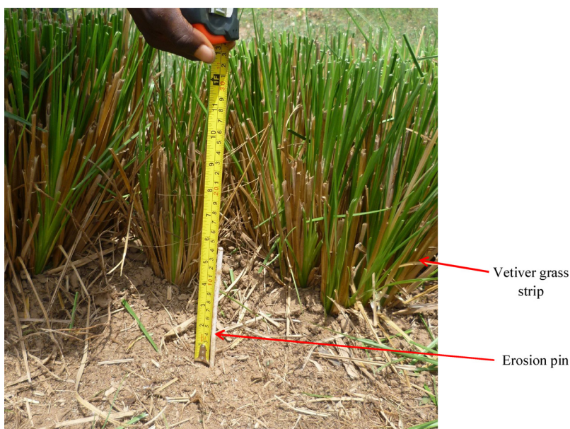
Fig. 1. Measurement of soil loss with erosion pin.
