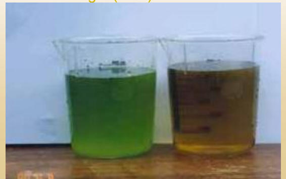
Vetiver cleaned up blue green algae in four days (left) sewage effluent containing high Nitrate (100 mg/L) and Phosphate (10 mg/L). (Right) sewage effluent after four days: VS reduced N level to 6 mg/L (94%) and P to 1 mg/L (90%).
