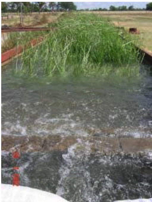
Photo 4 Left , very deep, turbulent flow at inlet flattened the first row. Below , note the calm water and very low water level behind last vetiver hedge
