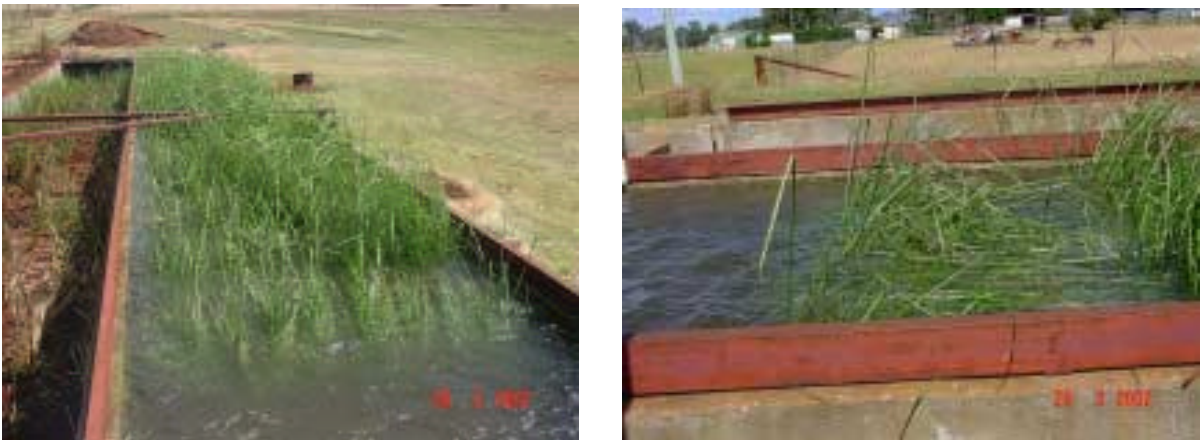
Photo 3 Test flow up to full depth of 60 cm showing the stiffness of the young vetiver stems
