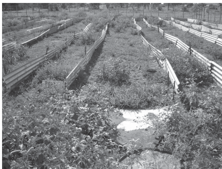
Figure 2 Experimental setup of the runoff plots.
