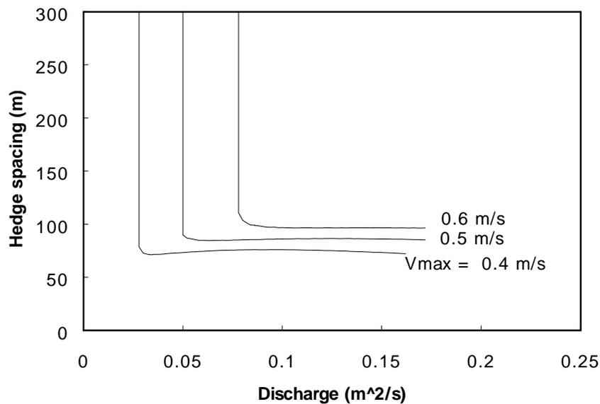
**Figure 7:** Effect of maximum permissible velocity on hedge spacing for a slope of 0.5% and Manning  $n$  of 0.03
