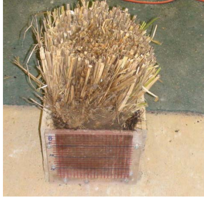
Figure 12: Vetiver stems after erosion testing
