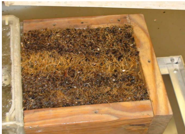
Figure 13: Vetiver roots after erosion testing
