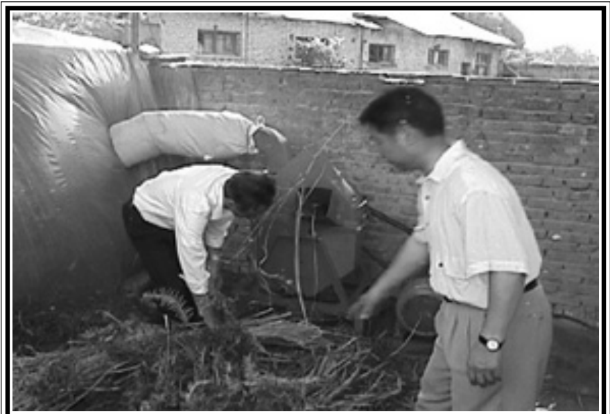
Dry vetiver grass leaves being fed through a hammer miller and collected in large bag on left for future use as a substrate for mushroom growing. This technology has potential in other countries as an enterprise for small farmers.
