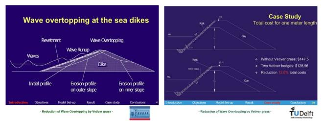
**Fig.1:** (Left) Erosion profiles of outer and inner dike batter. (Right) Reduction of crest height and construction cost when protected by 2 rows of vetiver.
