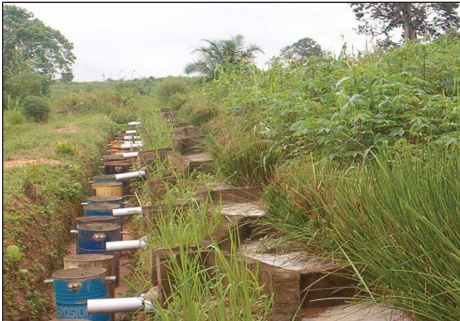
Figure 2 Sedimentation drums installed in a trench dug at the lower end of the erosion plot.
