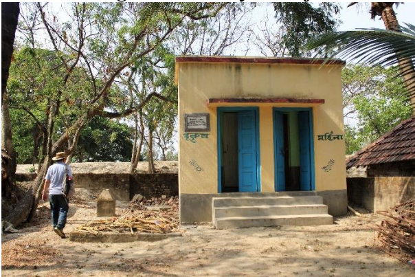
Village Community toilet front and back, discharge effluent to village pond
