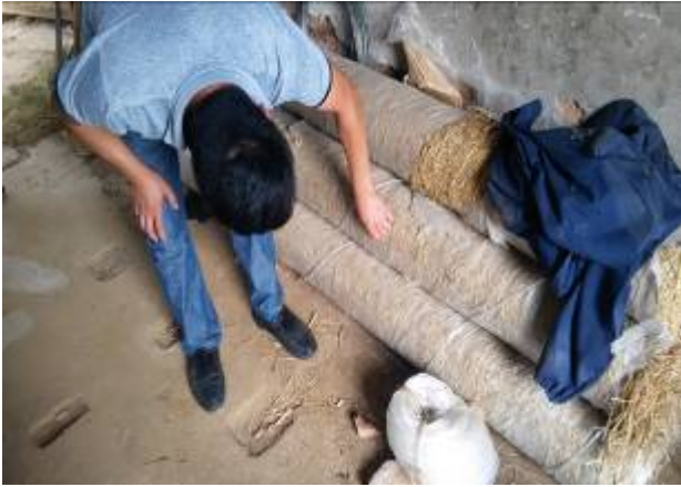
Photo 14 Vetiver mat for slope stabilization
